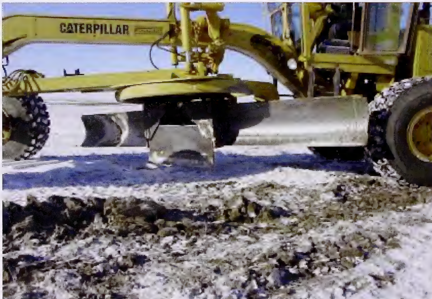
Photo 51 Step blade mounted on a grader.
